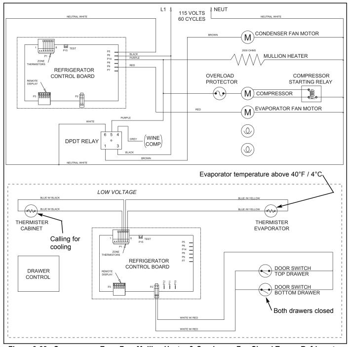
Figure 3-66. Compressor, Evap Fan, Mullion Heater & Condenser Fan Signal Trace, Refrigerator Section Calling for Cooling w/ Evaporator temperatures above 40°F / 4°C
