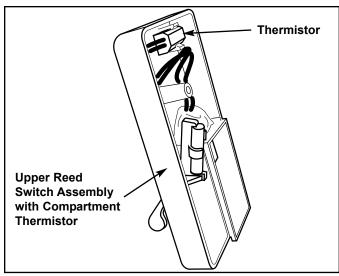
Figure 6-56. 427R Refrigerator Compartment Thermistor / Reed Switch
