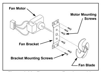
Figure 6-22. Evaporator Fan Assembly
