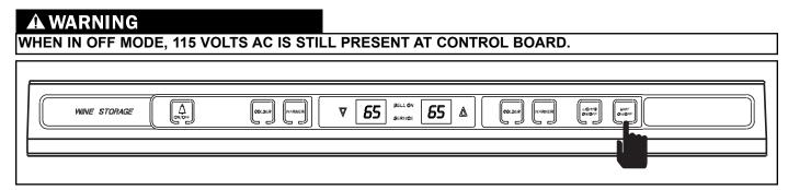
Figure 3-6. Unit ON/OFF, Press UNIT ON/OFF Key
