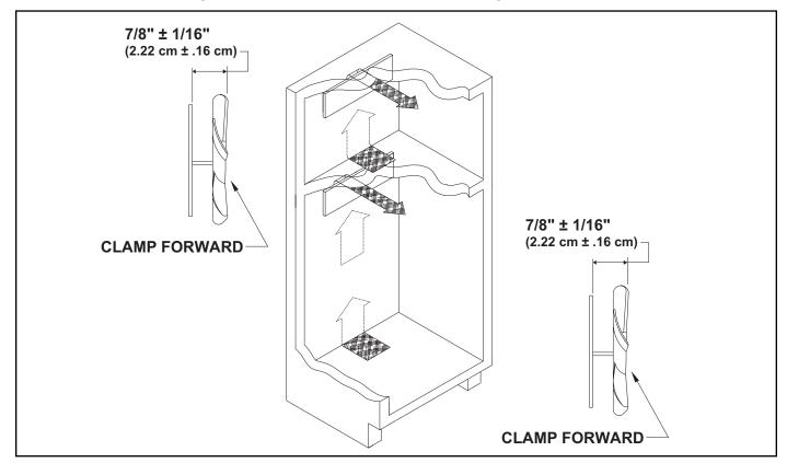
Figure 5-4. Air Flow & Fan Blade Spacing - Model 430
