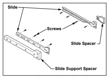
Figure 6-77. Cabinet Slide, Slide Support Spacer & Slide Spacer Removal
