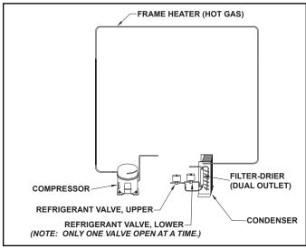
Figure 4-3. Refrigerant Valve(s)
