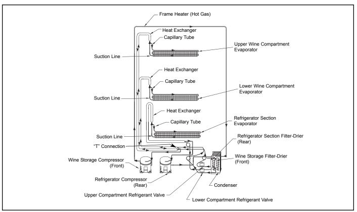
Figure 4-15. Model 427R Refrigerant Flow
