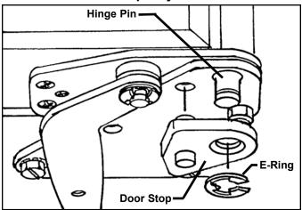
Figure 2-13. Model 430 Door Stop Installation
