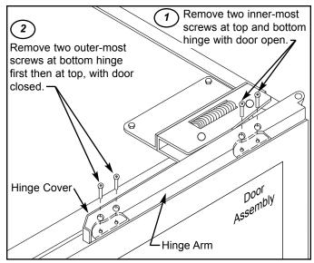
Figure 6-30. Door Assembly Removal
