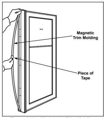
Figure 2-23. Model 430 Trim Molding Removal
