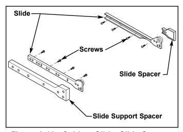
Figure 6-10. Cabinet Slide, Slide Support Spacer & Slide Spacer Removal
