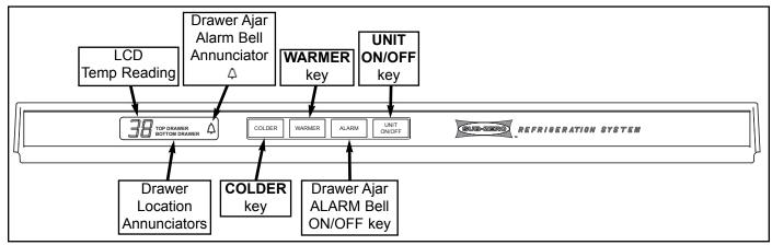
Figure 3-57. Model 427R Refrigerator Control Panel Layout, Prior to Serial #1728753
