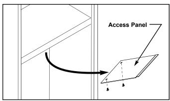
Figure 6-81. Control Board Access Panel
