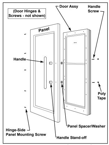
Figure 2-22. Model 430 Stainless Steel Door Panel Removal
