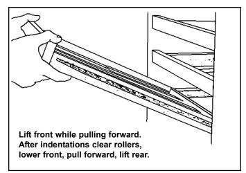
Figure 6-37. Wine Rack Assembly Removal
