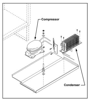
Figure 6-63. Compressor(s) & Condenser
