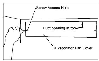
Figure 6-44. Evap Fan Cover Removal
