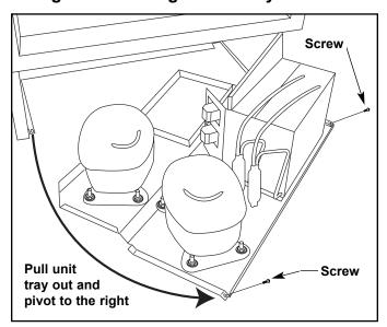
Figure 6-34. Unit Tray Removal
