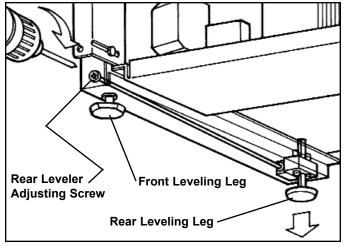
Figure 2-6. Model 427, 427R Adjusting Rear Leveling Leg
