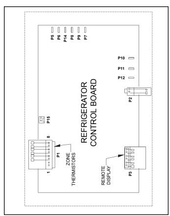
Figure 3-55. Model 427R Refrigerator Control Board Layout
