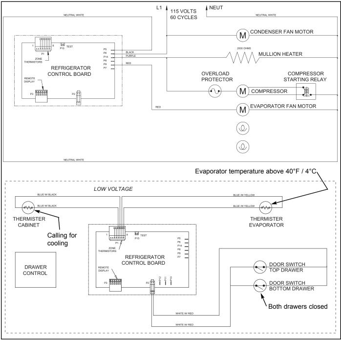
Figure 3-65. Compressor, Evap Fan, Mullion Heater & Condenser Fan Signal Trace, Refrigerator Section Calling for Cooling w/ Evaporator temperatures above 40°F / 4°C
