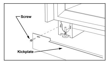
Figure 6-64. Kickplate Removal
