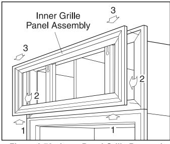
Figure 6-70. Inner Panel Grille Removal
