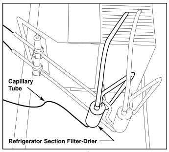
Figure 6-62. 427R Refrigerator Filter-Drier
