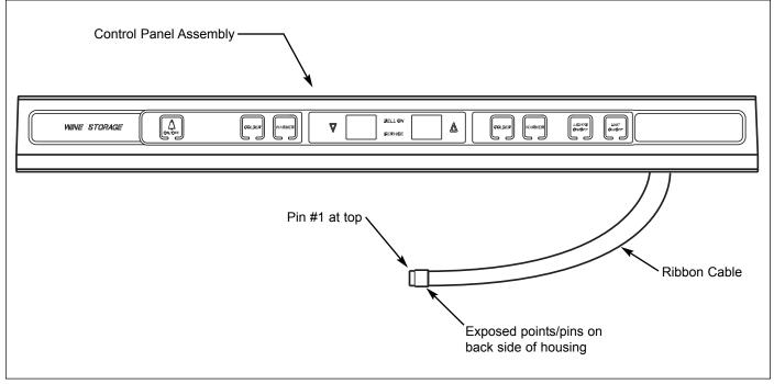
Figure 8-1. Membrane Switch
