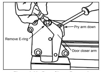
Figure 6-66. Door Closer Removal
