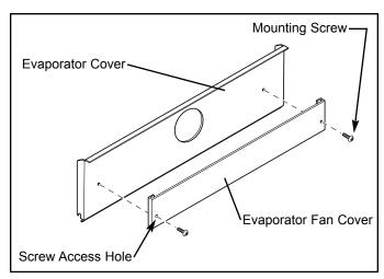
Figure 6-12. Evap Fan Cover Removal
