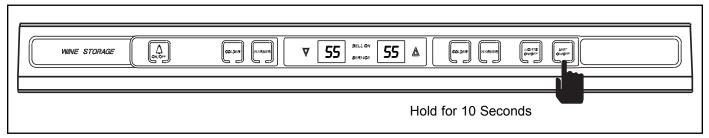
Figure 3-21. Initiate Sabbath Mode, Press and Hold UNIT ON/OFF Key for Ten Seconds
