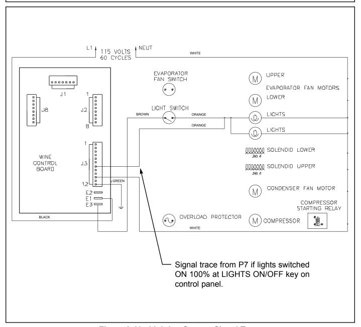
Figure 3-11. Lighting System Signal Trace
