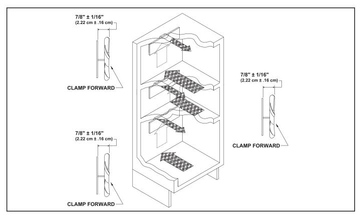
Figure 5-3. Air Flow & Fan Blade Spacing - Model 427R
