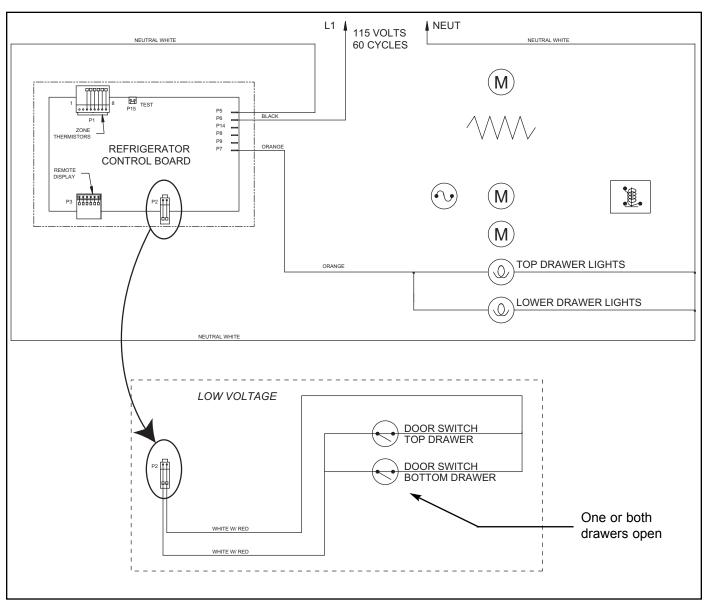
Figure 3-63. Model 427R Refrigerator Lighting System Signal Trace
