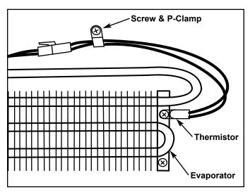
Figure 6-21. Evaporator Thermistor
