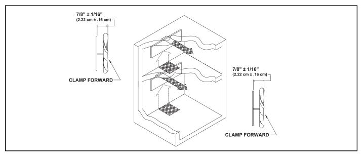
Figure 5-1. Air Flow & Fan Blade Spacing - Model 424
