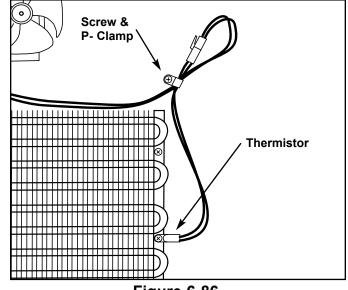
Figure 6-86. Evaporator Thermistor
