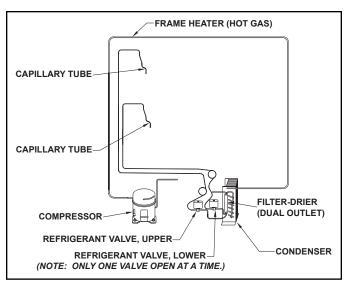
Figure 4-4. Capillary Tube(s)
