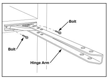
Figure 6-33. Hinge Assembly Removal
