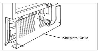
Figure 2-3. Model 427, 427R Kickplate/Grille Removal
