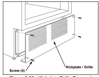
Figure 6-28. Kickplate/Grille Removal
