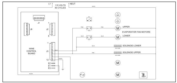
Figure 3-13. Evaporator Fan Power Signal Trace, Starting with Serial #1944319
