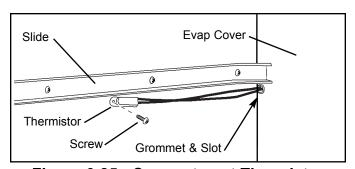
Figure 6-85. Compartment Thermistor
