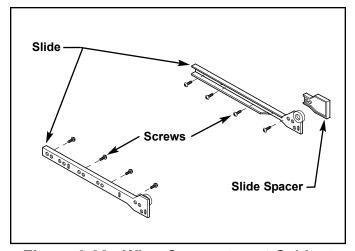
Figure 6-38. Wine Compartment Cabinet Slide & Slide Spacer
