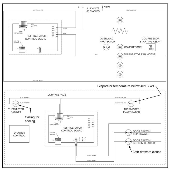
Figure 3-64. Evaporator Fan Power Signal Trace
