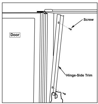
Figure 2-21. Model 430 Hinge-Side Trim Removal
