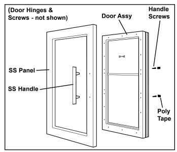
Figure 2-16. Model 424 Stainless Steel Door Panel Removal
