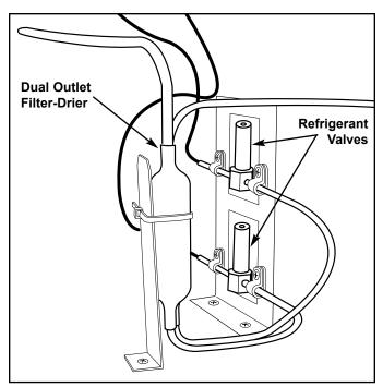
Figure 6-89. Capillary Tubes, Refrigerant Valves, Dual Outlet Filter-Drier
