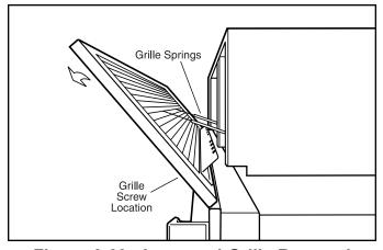
Figure 6-69. Louvered Grille Removal
