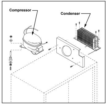
Figure 6-90. Compressor and Condenser
