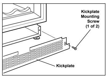
Figure 6-1. Kickplate Removal
