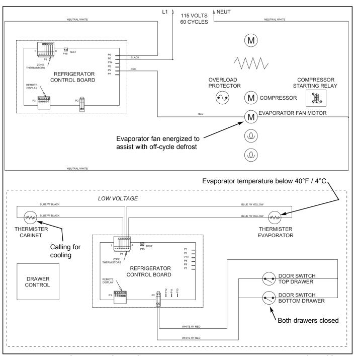
Figure 3-67. Cooling is Called for, but Evaporator Temperature is Below 40°F / 4°C, Compressor Waits for Evaporator to Fully Defrost
