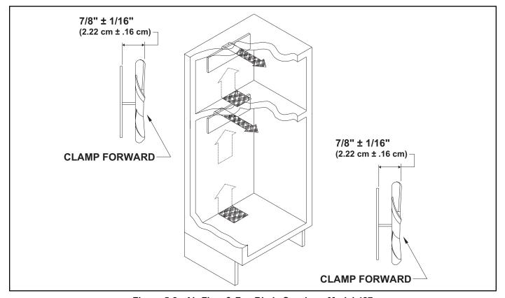
Figure 5-2. Air Flow & Fan Blade Spacing - Model 427
