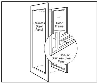
Figure 2-18. Model 427, 427R Door Panel Removal
