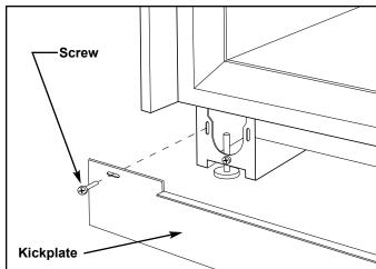
Figure 2-7. Model 430 Kickplate Removal
