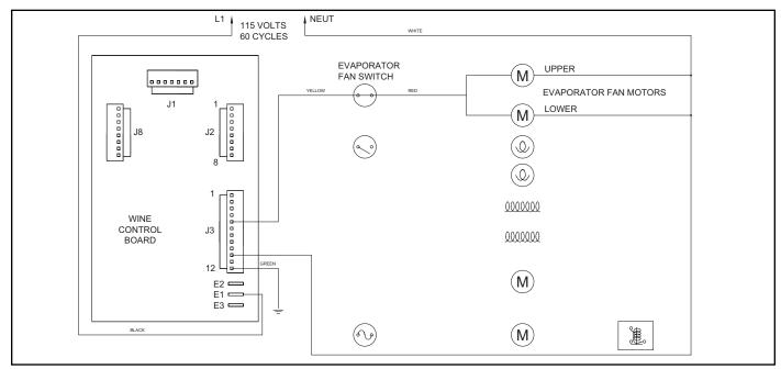
Figure 3-12. Evaporator Fan Power Signal Trace, Prior to Serial #1944319
