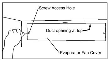
Figure 6-78. Evap Fan Cover Removal
