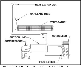
Figure 4-12. Suction Line & Heat Exchanger
