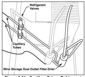
Figure 6-61. Capillary Tubes, Refrigerant Valves, Dual Outlet Filter-Drier
