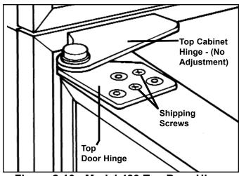
Figure 2-10. Model 430 Top Door Hinge
