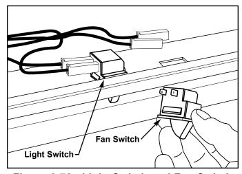
Figure 6-72. Light Switch and Fan Switch
