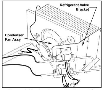
Figure 6-35. Condenser Fan Assembly
