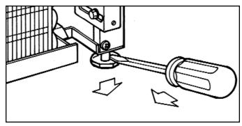
Figure 2-5. Model 427, 427R, 430 Adjusting Front Leveling Legs (427 Shown)
