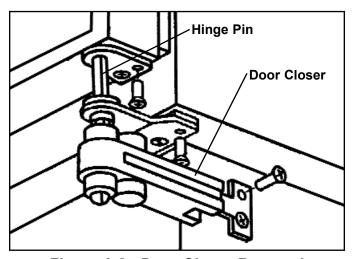
Figure 6-2. Door Closer Removal
