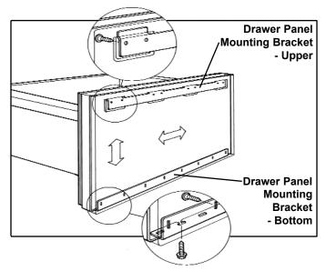
Figure 2-19. Model 427R Drawer Panel Removal
