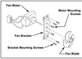
Figure 6-58. Evaporator Fan Assembly
