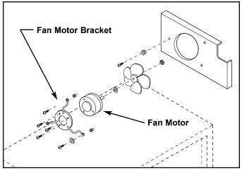
Figure 6-73. Condenser Fan Assembly
