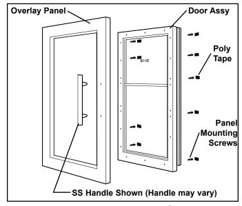
Figure 2-17. Model 424 Overlay Door Panel Removal
