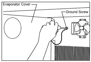
Figure 6-79. Evaporator Cover Removal
