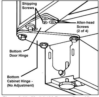
Figure 2-11. Model 430 Bottom Door Hinge
