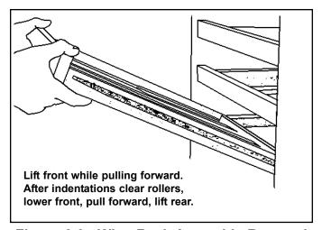
Figure 6-9. Wine Rack Assembly Removal
