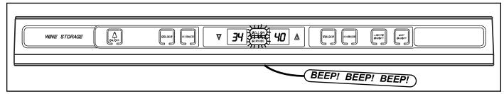
Figure 3-30. Cold Temperature Alarm with BELL ON Feature Enabled, "SERVICE" and "BELL ON" Flashing with Audible Alarm Beeping
