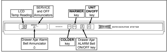
Figure 3-58. Model 427R Refrigerator Control Panel Layout, Starting with Serial #1728753
