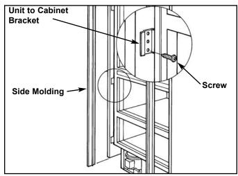
Figure 2-4. Model 427, 427R Molding Strip & Bracket
