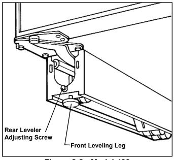
Figure 2-8. Model 430 Adjusting Rear Levelers
