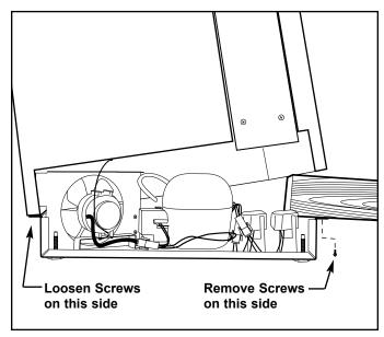
Figure 6-8. Unit Tray Component Access
