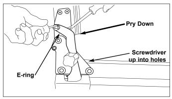
Figure 2-20. Model 430 Detaching Door Closer
