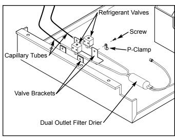
Figure 6-25. Capillary Tube, Refrigerant Valve, Filter-Drier
