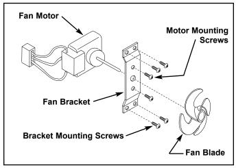
Figure 6-87. Evaporator Fan Assembly
