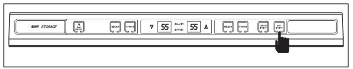
Figure 3-22. Exit Sabbath Mode, Press and Release UNIT ON/OFF Key
