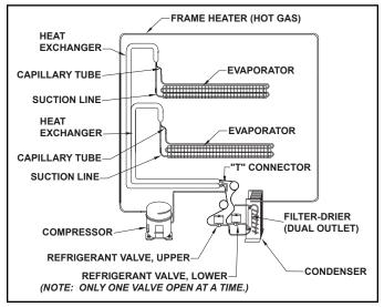
Figure 4-6. Suction Line(s) & Heat Exchanger(s)
