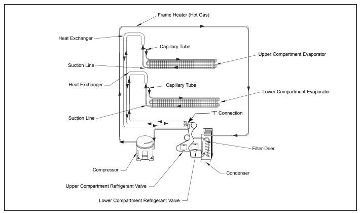
Figure 4-13. Model 424 Refrigerant Flow
