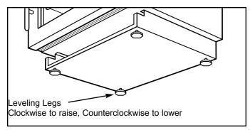
Figure 2-1. Model 424 Leveling Legs
