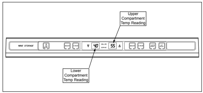
Figure 3-10. Temperature Display (Shown in degrees Fahrenheit)
