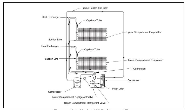
Figure 4-14. Model 427 Refrigerant Flow
