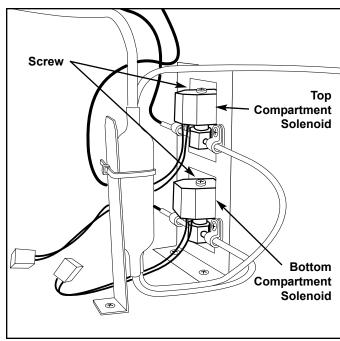
Figure 6-74. Refrigerant Solenoid Valves
