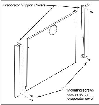
Figure 6-47. Refrigerator Evaporator Support Cover Removal
