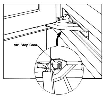
Figure 2-12. Model 427, 427R Door Stop Adjustment
