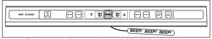
Figure 3-27. Warm Temperature Alarm with BELL ON Feature Enabled, "SERVICE" and "BELL ON" Flashing with Audible Alarm Beeping
