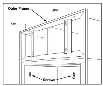
Figure 6-71. Outer Panel Grille Removal
