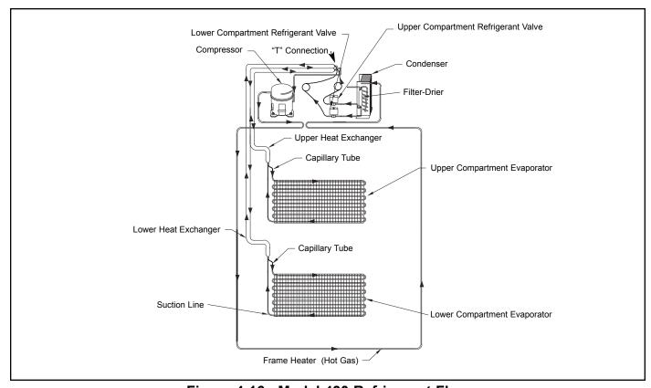
Figure 4-16. Model 430 Refrigerant Flow
