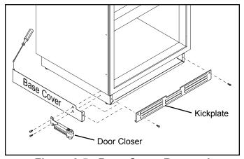
Figure 6-5. Base Cover Removal
