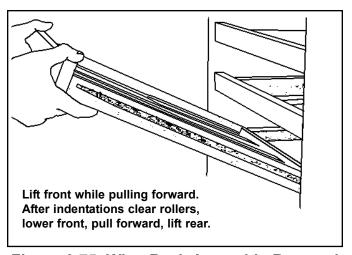
Figure 6-75. Wine Rack Assembly Removal
