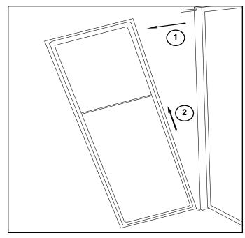
Figure 6-68. Door Assembly Removal
